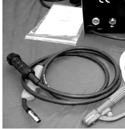
Image 2b MIG gun "Euro" style with electrode holder
